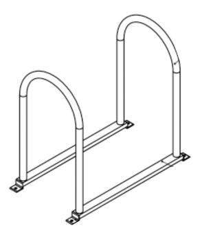
The bicycle racks available through this grant are shaped like the rack pictured above. The finish of the rack is black powder coat. Each loop accommodates two bicycles. The grant offers any combination of two-loop (pictured), threeloop, and four-loop racks.
