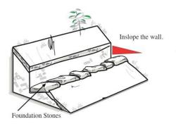
Figure 7: Rock Retaining Wall
